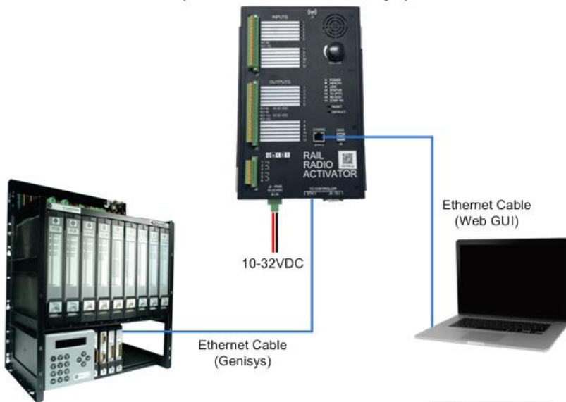
RRA Connection Diagram (ELX to RRA via Genisys)
